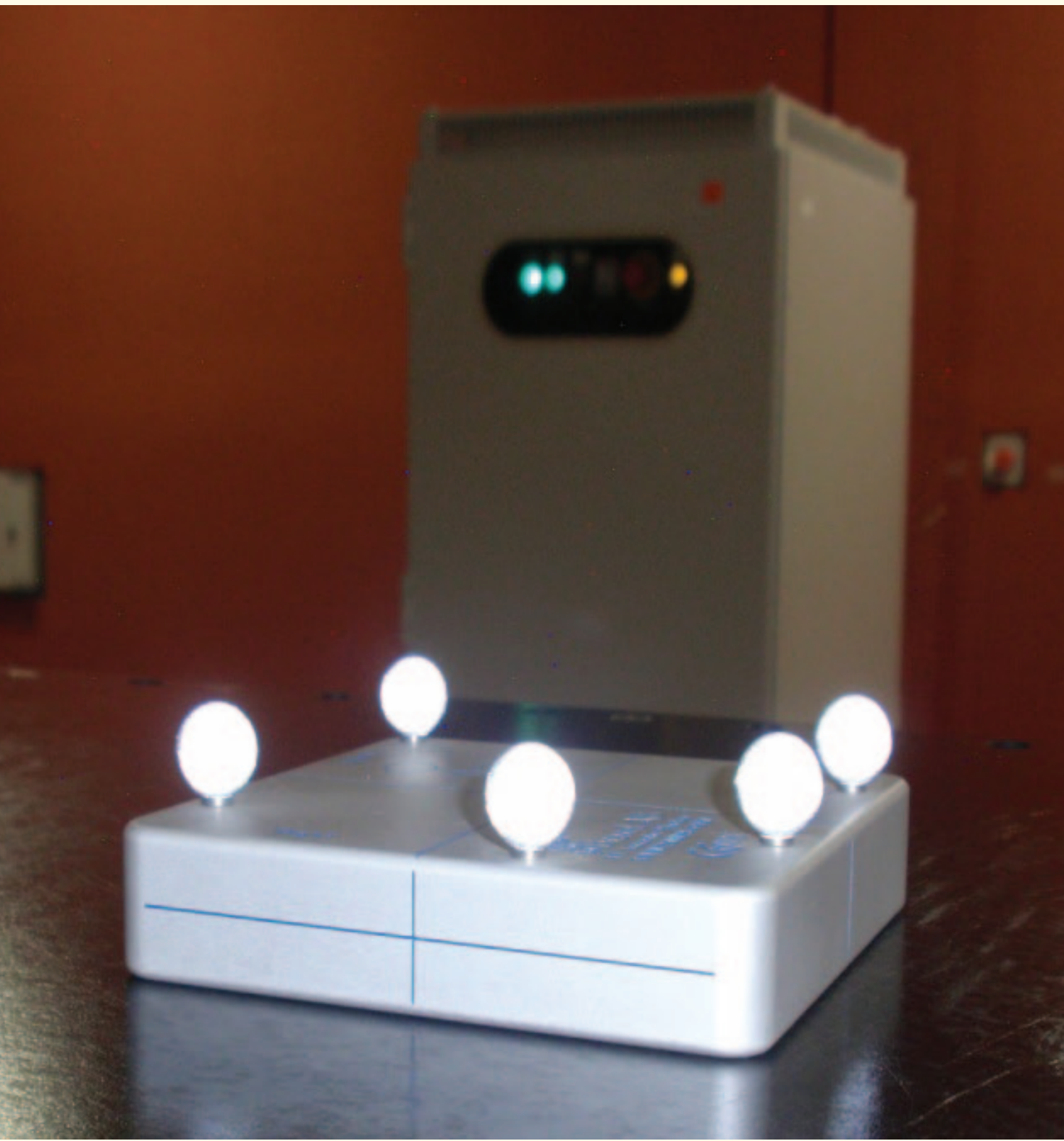
Aligns couch top with machine isocentre
