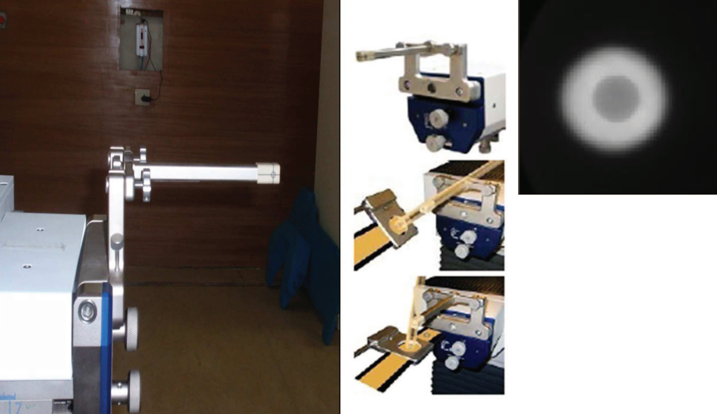
Ensures accuracy of Laser with isocentre of Gantry, Collimator and Table. Deviation <0.7 mm acceptable.
