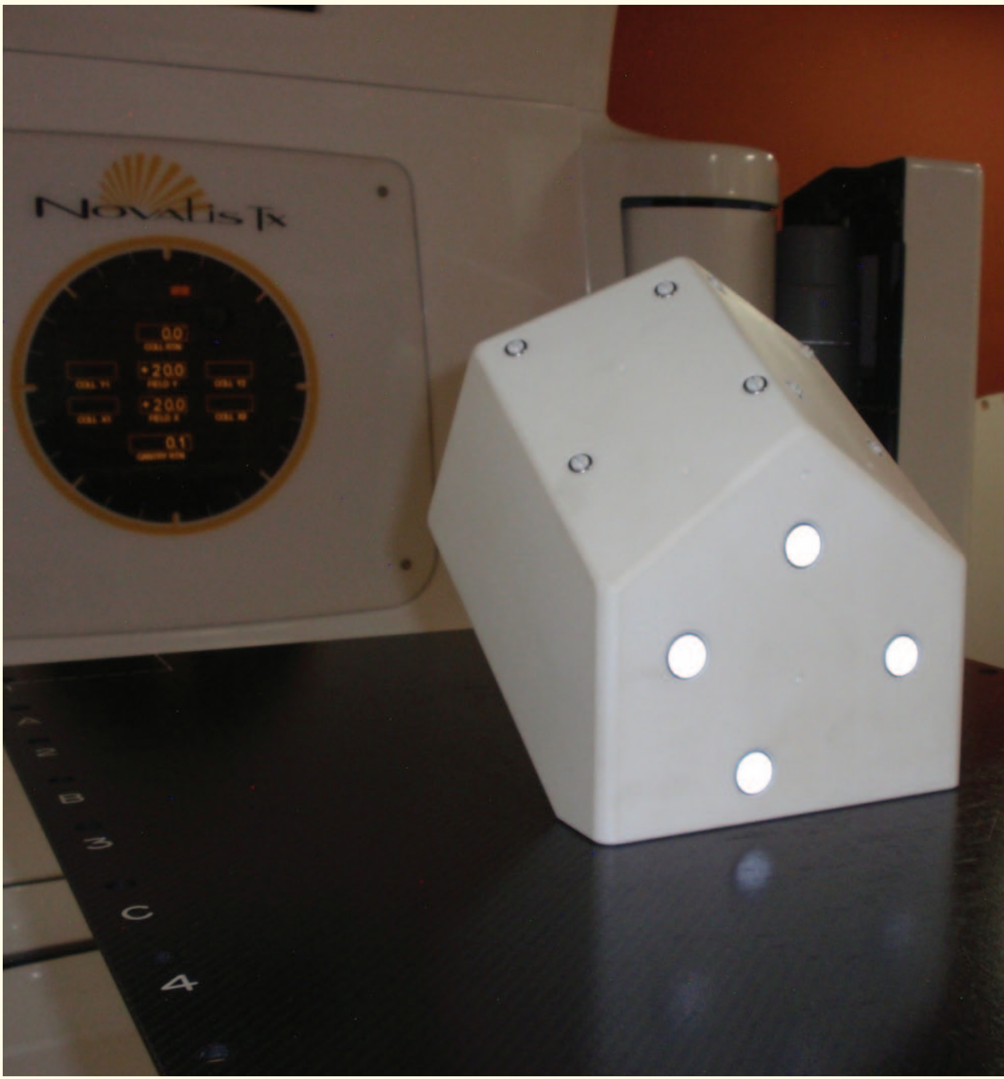
Ensures that the central axis of the X-ray beam passes through the machine isocenter
